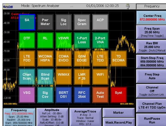
Figure 3: UCTT feature selection after pressing the MODE button.
