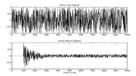
Figure 1: A hypothetical Echo Sounder test signal (top) and returned echo signal (bottom).
