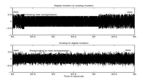
Figure 4: Rate renegotiation signal sequence. In this example, the downstream uses V90 mode. If V34 modem were chosen, the signal flow on top would look different (similar to that at the bottom).
