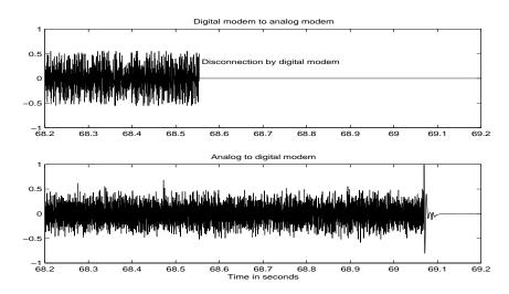
Figure 5: An actual example of the modem disconnection sequence.
