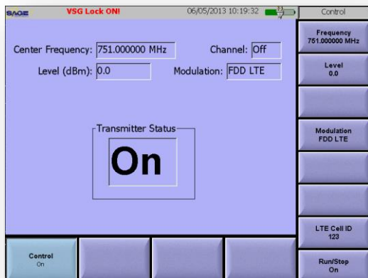
Figure 1 & Figure 2 Show the Vector Generator Mode (VSG) with FDD-LTE SigGen turned “On” [0.0 dBm, 751 MHz, with PCI of “123”]. In Figure 2 , the RfOut port was looped to the RFin and Mode was switched to Power Meter to display signal.
